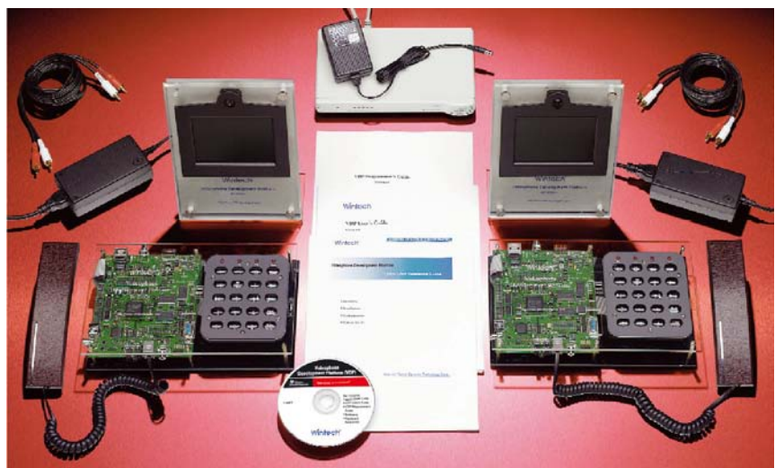
Each VDP is comprised of two DSP based boards, two DSP-based boards, two CCD cameras, two 5-inch LCD displays, two phone keypads as well as the software and documentation to get started immediately.
